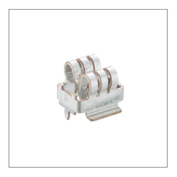
High-current contact bush with positioning pegs, mateable from top or bottom direction, for tab contacts 1.5–2.0 mm, for printed circuit boards or lead frames
